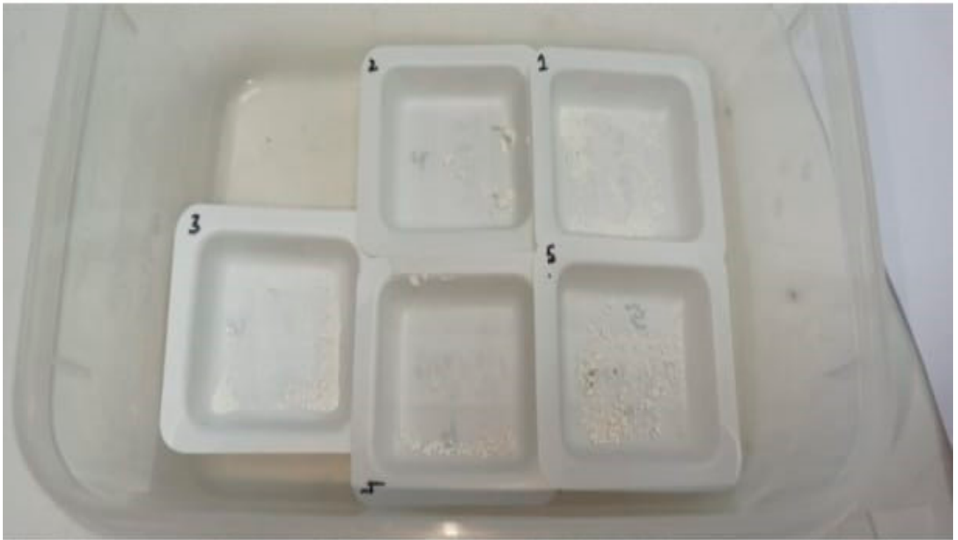
Figure 1. Crushed samples of the five root canal sealers.
