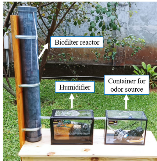
Fig. 5 Completed biofilter model
