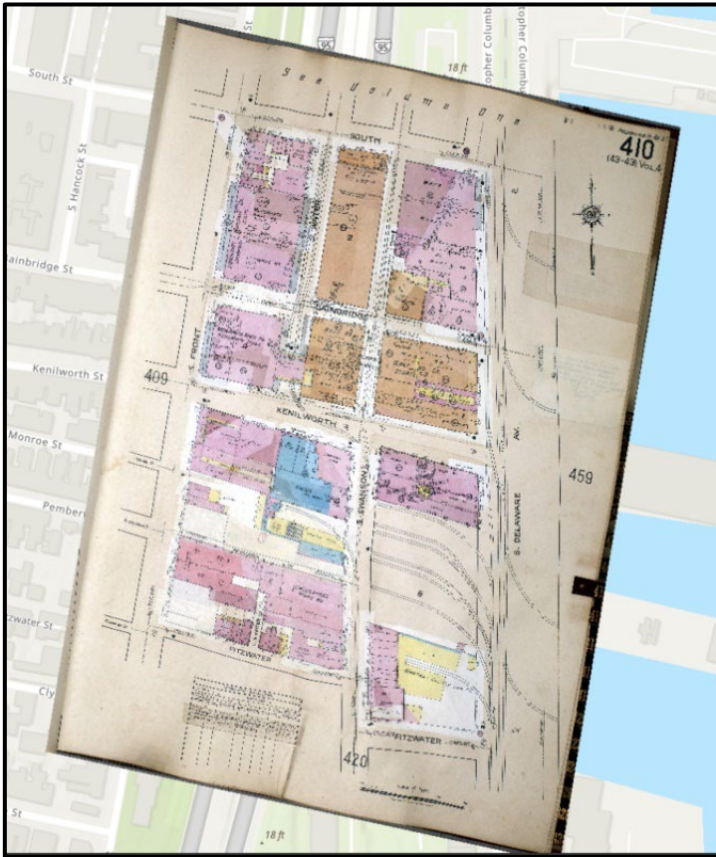
Figure 12. Colorized Sanborn map used to extract the building materials.
