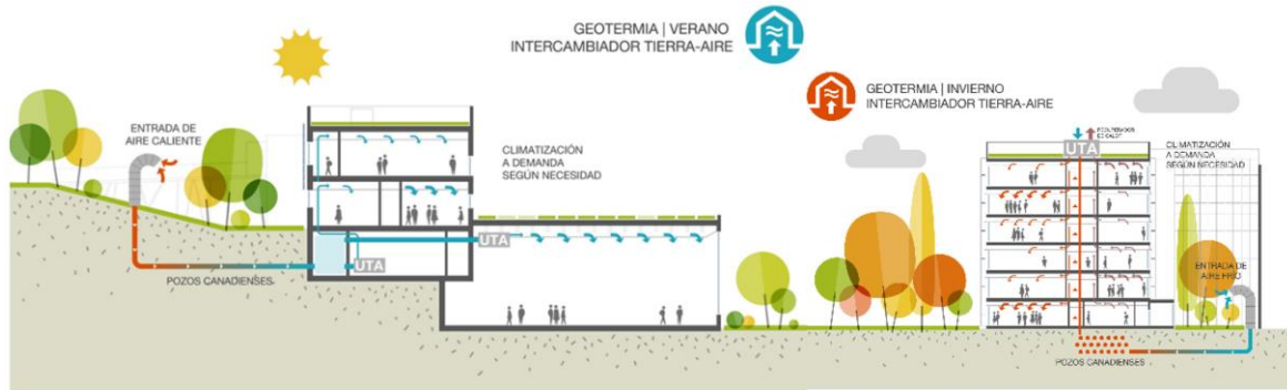
Figure 2. Climate control through Canadian wells at the Soria Campus and the IndUVa building at Valladolid.
