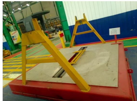
Gambar 5. Test stand wheel boogie
