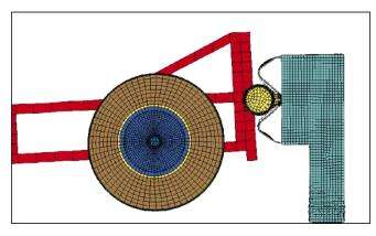
Figure 8: Dolly behaviour when contacted with the prototype model.
