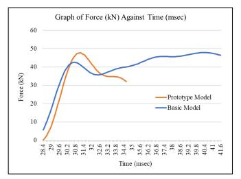
Figure 5: Comparison graph between existing w-beam and newly developed prototype.
