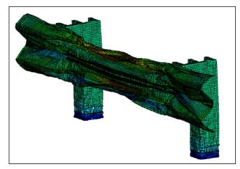
Figure 6: Existing w-beam model deformation.
