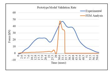
Figure 4: Validation accuracy graph of newly developed prototype.
