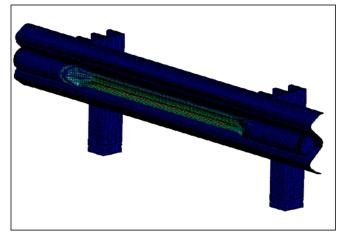
Figure 7: Newly developed prototype model deformation.
