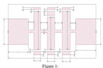
The top view of the layout for the low pass filter
