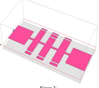
Figure 2: The 3D view of the low pass filter
