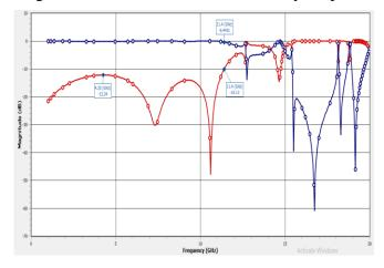
Figure 3: Result of the proposed low pass filter
