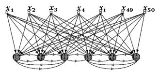
*Figure 6.* Architectural graph of a simple memory based learning network with feedforward (excitatory) connections from the source nodes to the neurons, and lateral (inhibitory) connections among the neurons; the lateral connections are signified by open arrows.
