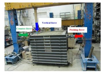
Fig. 2 The measuring principle of the multi-level shear box [8]
