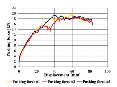
**Fig. 5** A typical shear graph (curve) with the three repetitions of the measurement (RB without geosynthetic reinforcement, shearing plane #2, i.e., 10 cm above the geosynthetics' theoretical plane)
