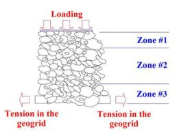
**Fig. 1** The zones of the interlocking effect in a granular material due to a planar geogrid layer (on the basis of [33,34])
