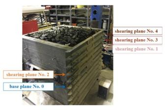
Fig. 3 Marking of shearing planes [8]
