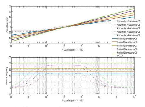
**Fig. 5** Frequency response of  $G_{3rd}(\gamma, \alpha)$  for  $\alpha = 0.5, 0.6, 0.7, 0.8, 0.9$  at  $\Delta = 0.001$  sec
