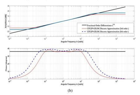
**Fig. 3** a) Frequency response of the realization using *z*-domain and  $\gamma$ -domain for  $\alpha = 0.4$  with  $\Delta = 0.001$  sec; b) Fréquency responses of *G* (*s*,0.4), *G*<sub>3rd</sub>( $\gamma$ ,0.4) and *G*<sub>5rd</sub>( $\gamma$ ,0.4) at  $\Delta = 0.001$  sec
