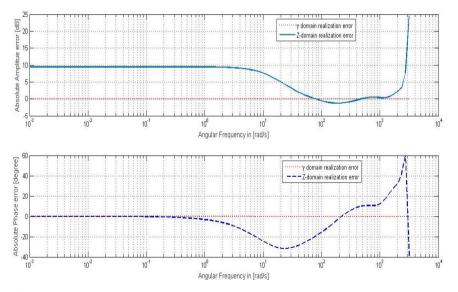
Fig. 4 Absolute errors between actual and approximated realization in z-domain and y-domain
