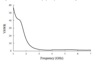
Fig. 4 Simulated VSWR versus frequency curve
