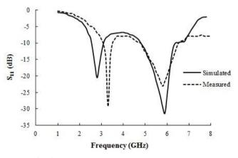
Fig. 9 Simulated and Measured return loss curve
