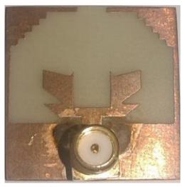
Fig. 7 Fabricated antenna
