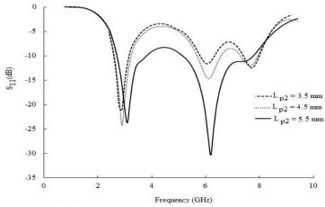
Fig. 3 Variation of return loss with patch length
