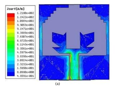
Fig. 5 Simulated Current density distribution curve (a) 2.8 GHz and (b) 5.9 GHz
