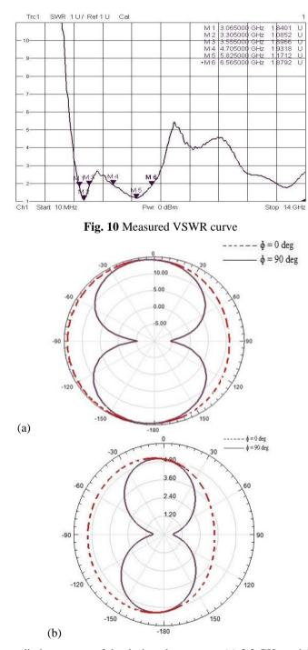
Fig. 11 The radiation pattern of the designed antenna at (a) 3.3 GHz and (b) 5.82 GHz
