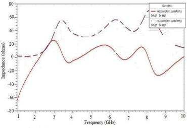
Fig. 6 Simulated input impedance response curve
