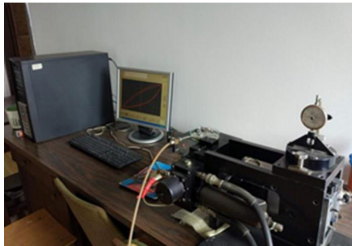
Fig. 1 DSSA in the laboratory for soil dynamics
