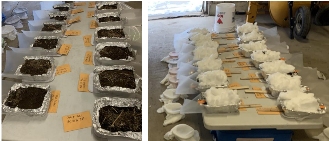
Fig. 4.5. Snowmelt-runoff study setup – initial setup shown on the left, with PRS® probes and added snow on the right. Aluminium containers and plastic sheets were used to funnel the runoff water into the containers using cheesecloth as a filter.
