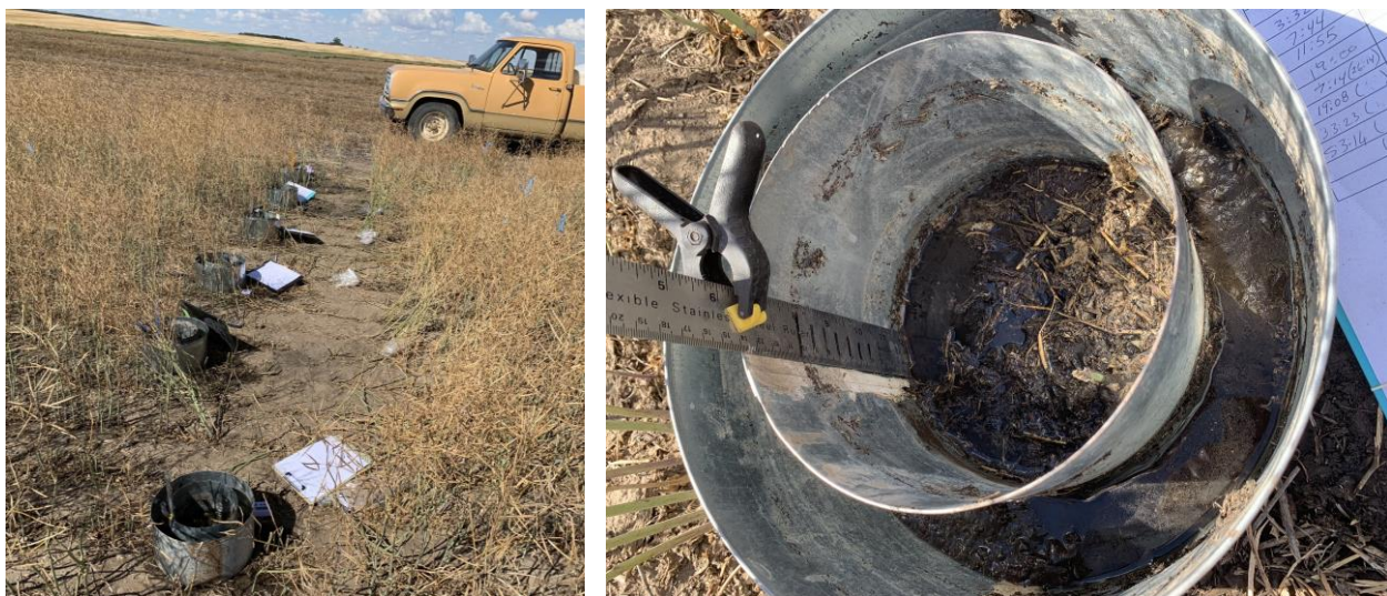
Fig. 4.4. Infiltration measurements in the field set up for each plot (left). A close-up of the setup (right) shows the water levels in both rings.
