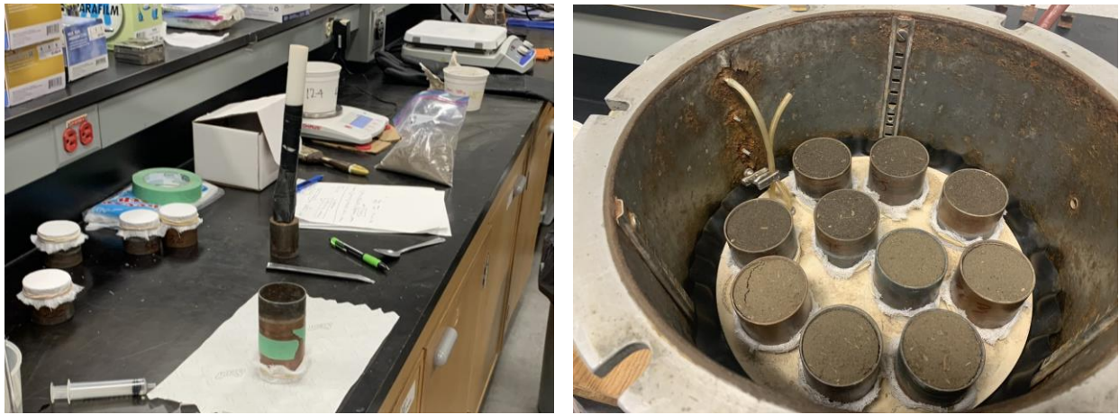
Fig. 3.2. Preparing soil moisture cans for the water holding capacity experiment (left) and moisture cans in the pressure plate apparatus (right).
