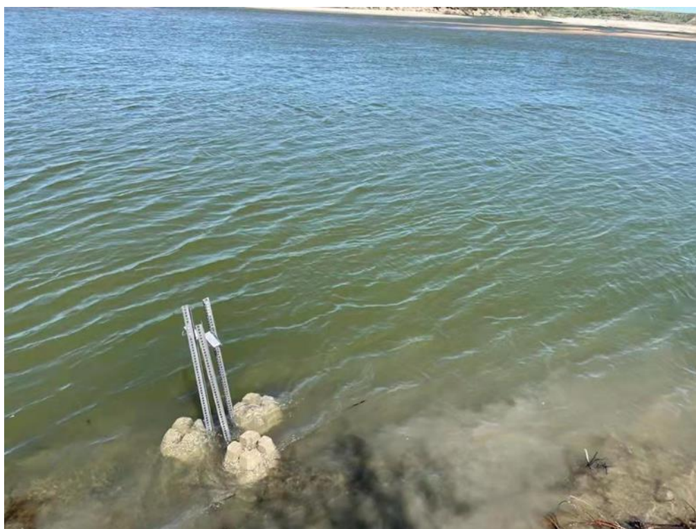
Figure A2 The setup for fixation of DGT sediment probes in the field.
