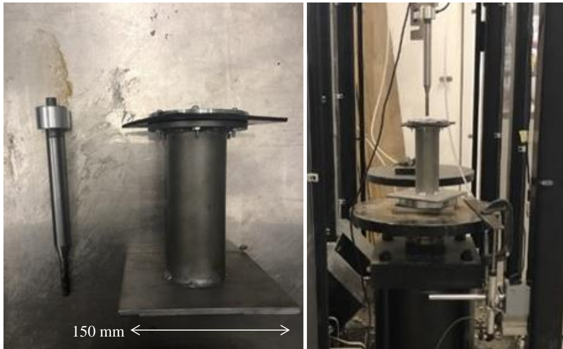
Figure 3.4 (Left) BGM mounted in Puncture Frame (Right) Puncture Apparatus in Load Frame
