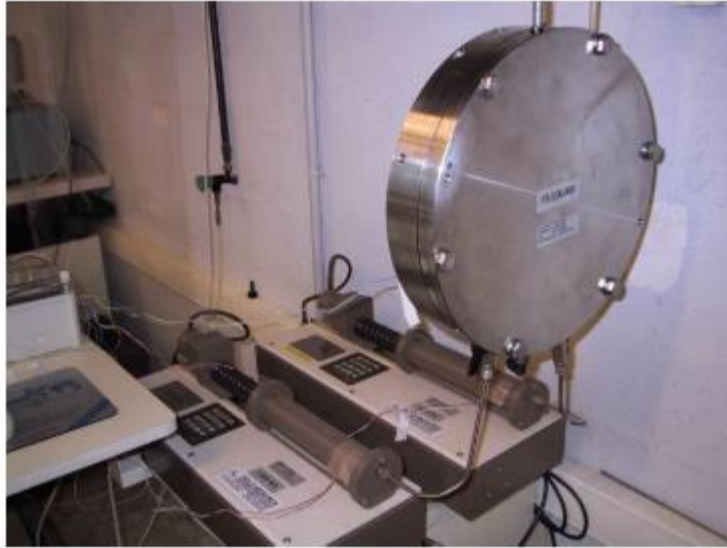
Figure 2.1 Stainless Steel Pressure Cell (Touze-Foltz et al. 2015)
