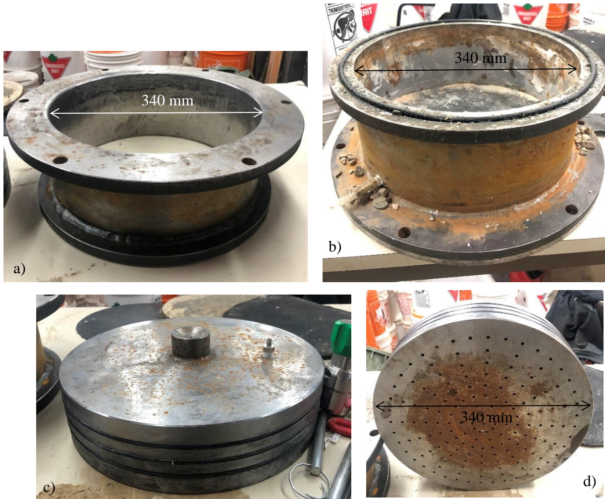
Figure 3.6 (a) Upper Body Assembly (b) Lower Body Assembly (c/d) Load Plate Assembly
