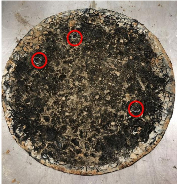
Figure 4.23 ES4 Sample with Significant Deformation (+20°C)
