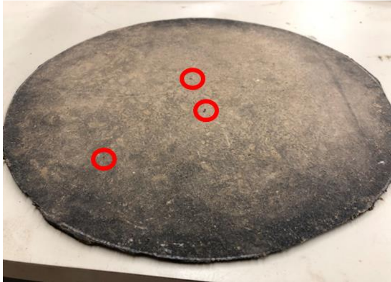
Figure 4.21 ES2 Sample with Significant Deformation Points (0°C)
