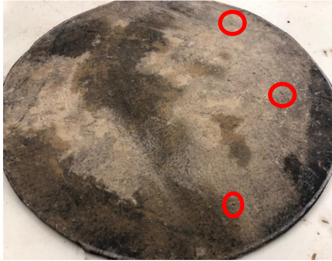
Figure 4.20 ES2 Sample with Significant Deformation Points (-15°C)
