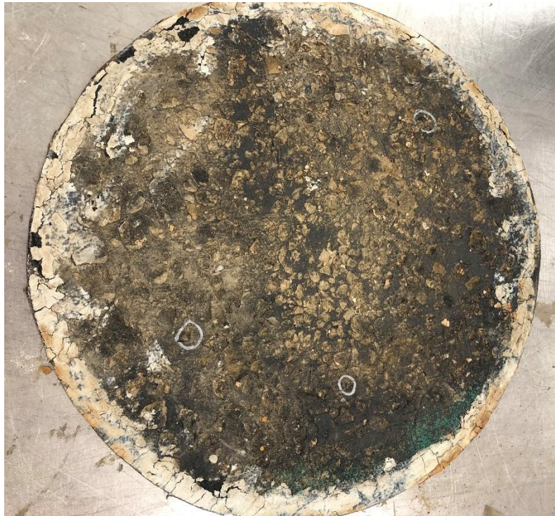
Figure 4.22 ES2 Sample with Significant Deformation (+20°C)
