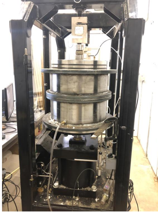
Figure 3.7 Full Load Assembly mounted in Air Frame
