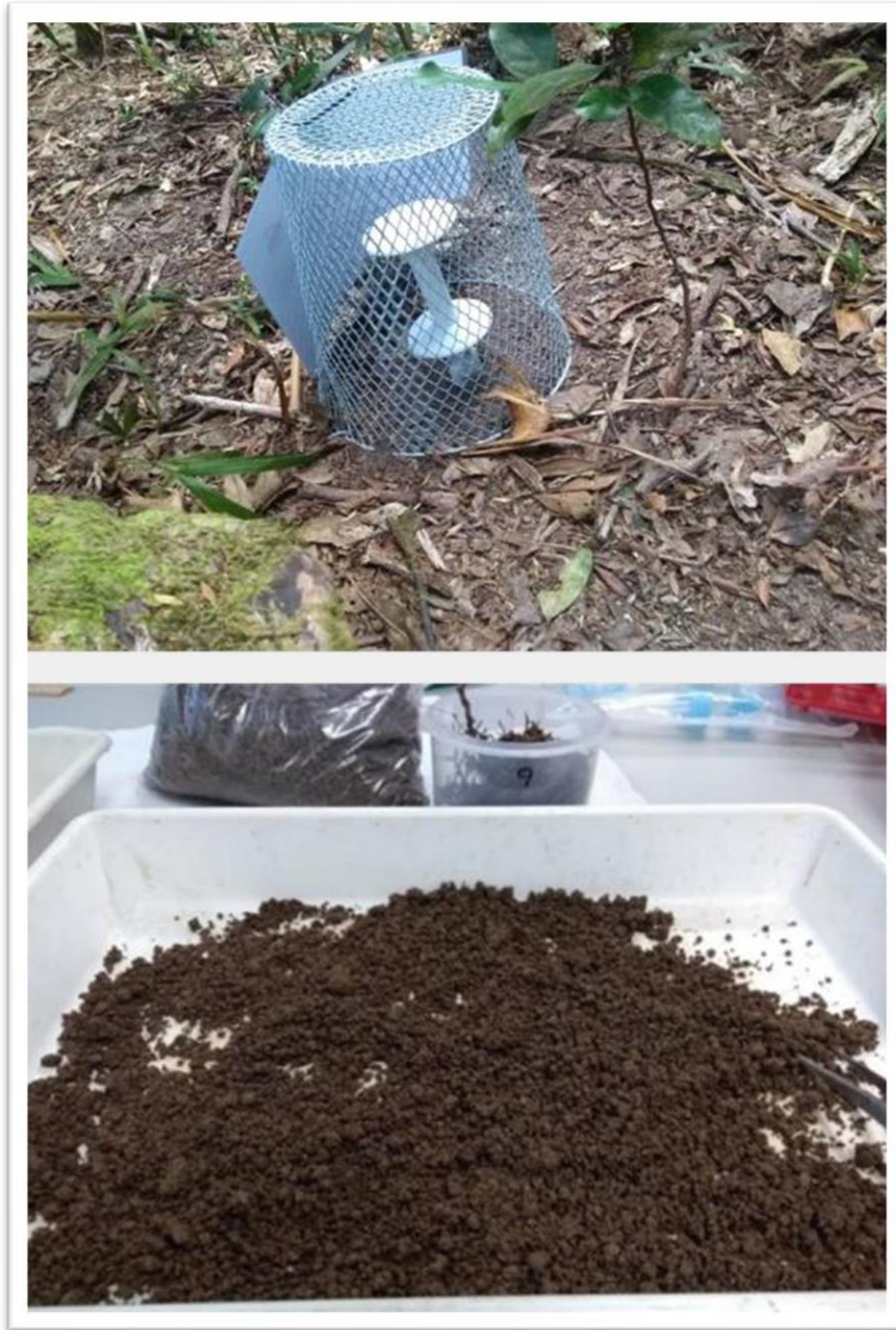
The Temperature and Soil Moisture Sensor (model TMS-4, TOMST, Prague, Czech Republic) recording microclimate from a study site (~1000 m a.s.l.) in the Australian Wet Tropics ( Top ); Soil sample collected from the same study site being processed in the laboratory ( Bottom ).
