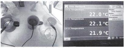
Picture 2 - Order of Cups both physically and on the data logger
