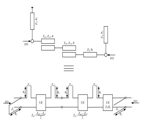
Figure 3. Schematic of *BPF*<sub>2</sub> with its equivalent circuit model.
