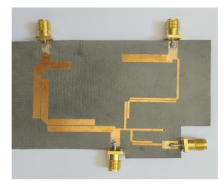
Figure 12. Fabricated prototype of proposed triplexer.
