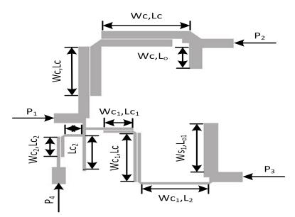
Figure 8. Layout model of proposed triplexer filter.
