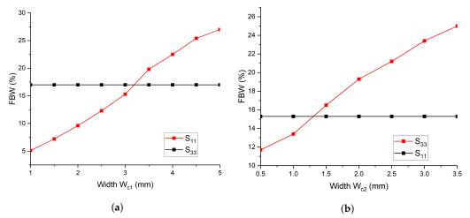
**Figure 5.** Frequency response with a variable width of coupled lines. (a) By Varing  $W_1$ ; (b) By Varing  $W_2$ .
