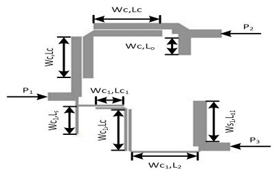
Figure 1. Layout model of proposed diplexer filter.
