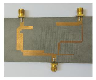
Figure 10. Fabricated prototype of proposed diplexer.
