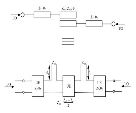
Figure 6. Schematic of *BPF*<sub>3</sub> with its equivalent circuit model.
