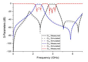
Figure 9. S-parameter response of proposed diplexer.
