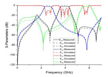
Figure 11. S-parameter response of proposed triplexer.
