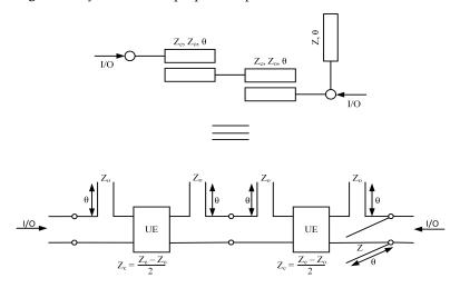
Figure 2. Schematic of *BPF*<sub>1</sub> with its equivalent circuit model.
