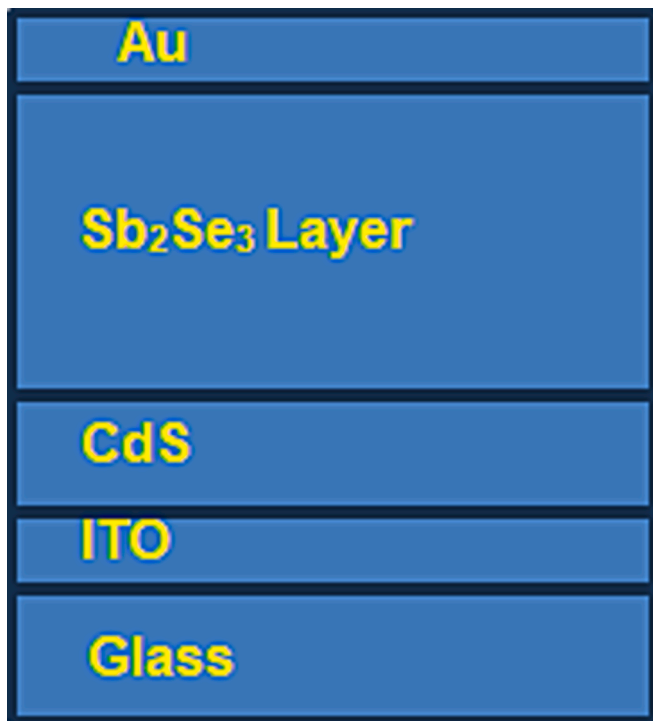
Fig. 1. The schematic structure of a cds/ sb 2 Se 3 thin film solar cell.
