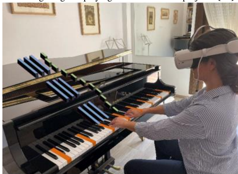
Fig.5. Photograph of a user playing the piano with the application and what she is seeing superimposed (blue and green) and the C keys (orange).
