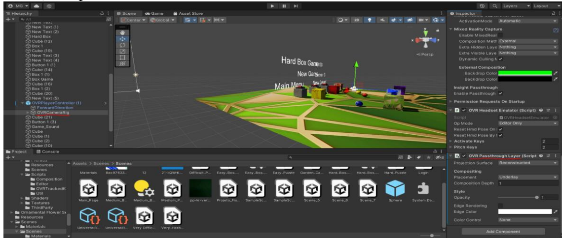
Fig.40. OVR Passthrough API Script and other Settings for Augmented Reality Implementation
