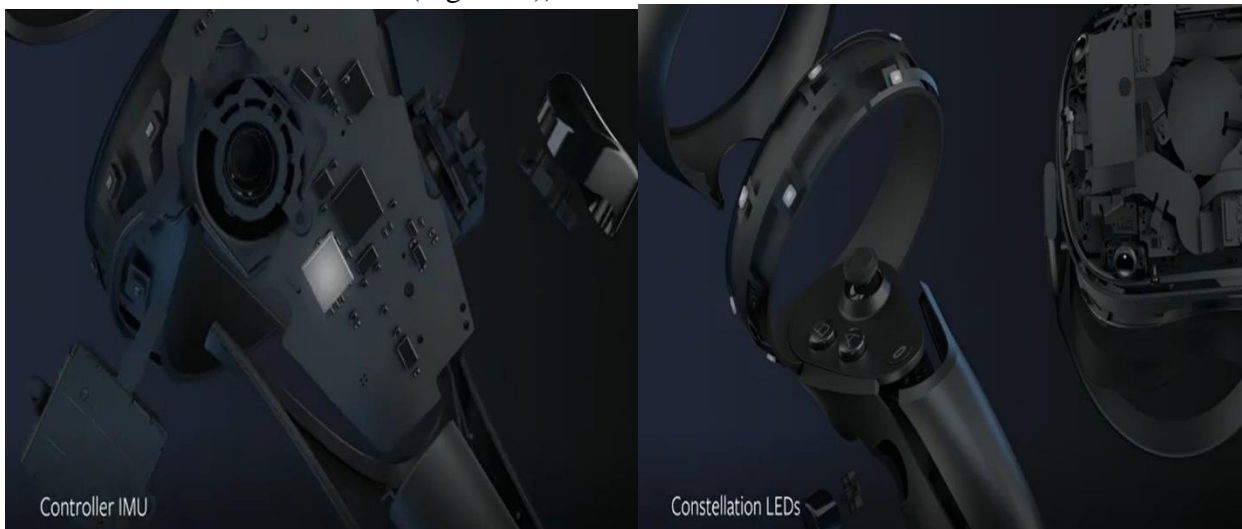
Fig.16. a) Controller IMU in the sensors hand commands b) Constellation LEDs in two sensors hand commands
