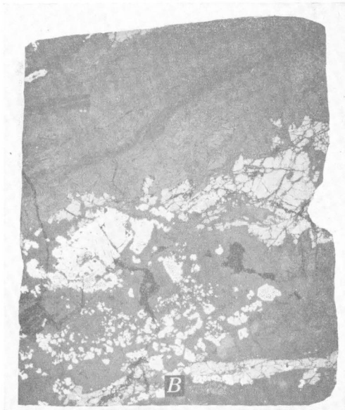
B. GALENA, SPHALERITE, CHALCOPYRITE, AND QUARTZ FILLING A FISSURE IN MANGANIFEROUS CARBONATE (GRAY, IN TOP THIRD AND ALONG BOTTOM EDGE). QUARTZ IN VEIN CONTAINS VUGS (BLACK). PATARA MINE.
