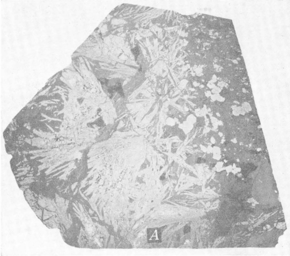
A. MARCASITE (BLADED) FILLING OPENINGS AND REPLACING A MIXTURE OF FINE-GRAINED PYRITE, SPHALERITE, GALENA, AND CHALCOPYRITE, ON LEFT. CALCITE (MEDIUM GRAY, ON RIGHT) IS LATER FISSURE FILLING. VUGS ARE BLACK. FRAY MARTÍN PROSPECT.
