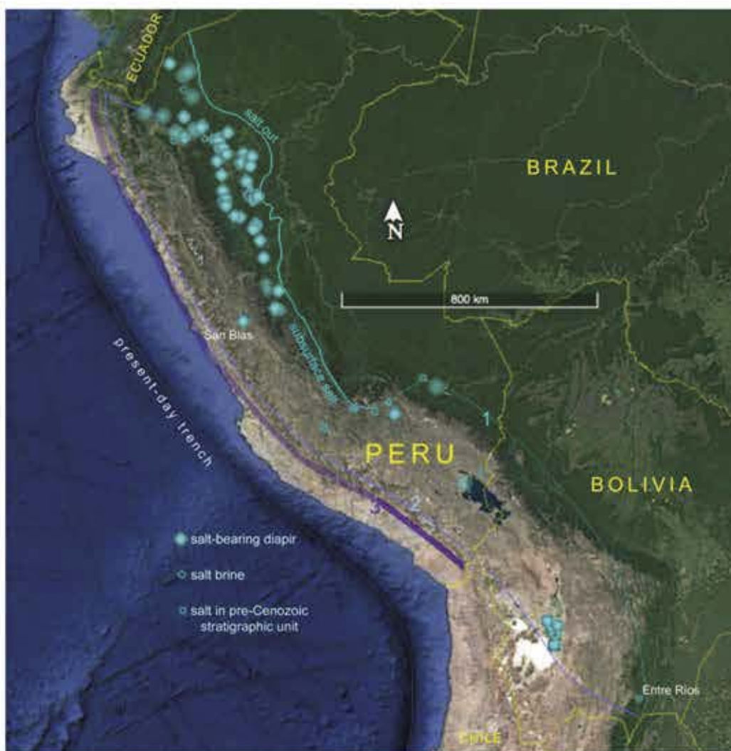
Figure 1. Outline of the possible extension of the salt basin, considering both autochthonous and allochthonous salt. Blurry symbols indicate an imprecise position. Line 1: eastern limit of autochthonous salt (hypothetical in southern part of map); line 2: hypothetical western limit of salt (which is expected to have been in part allochthonous); line 3: position of the magmatic arc during Pucará times (the actual arc was broader than the illustrated line); all lines are hypothetical where thin or blurry. This map does not show the other elements used to construct it, such as the numerous occurrences of other evaporites and the structural proxies detailed in text. This map suggests that the salt basin should be expected to extend into Ecuador, but no corresponding salt has been reported from this country so far (see Baby et al., 2014).
