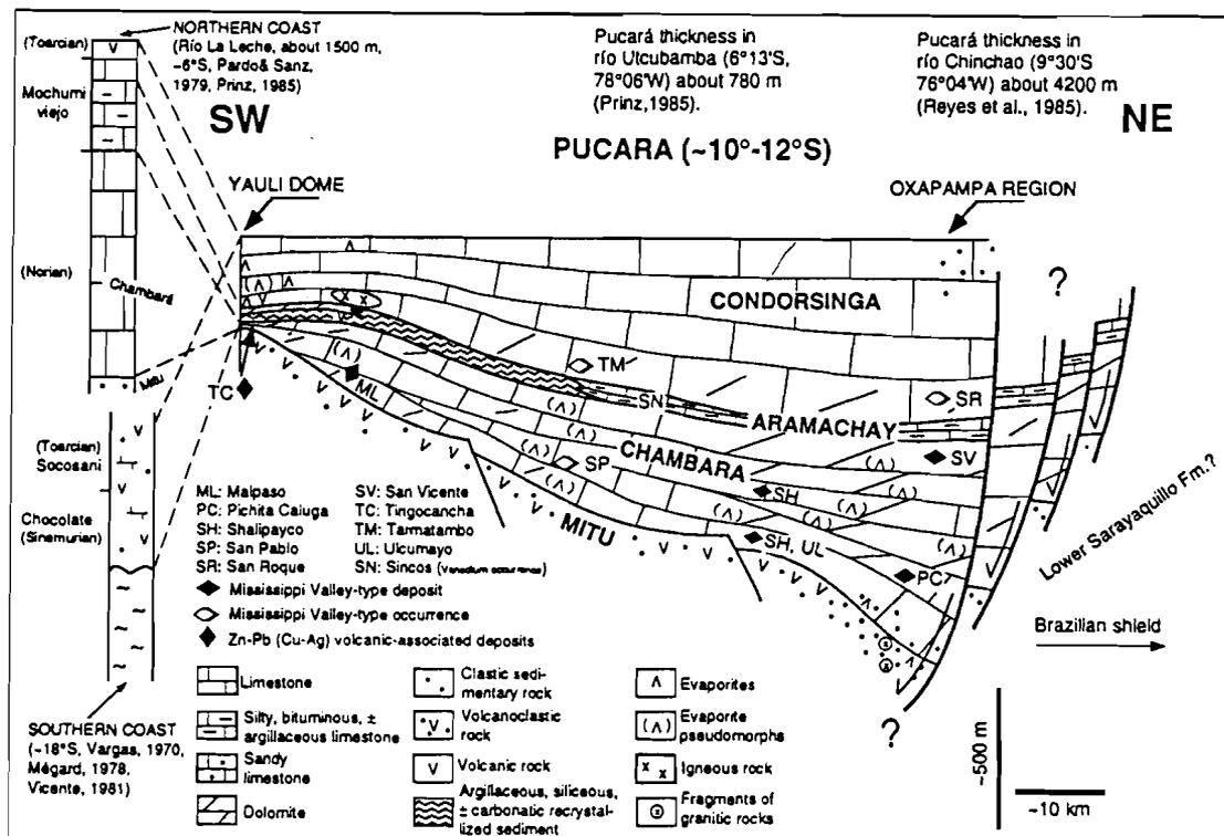
Fig. 2. Schematic section of the Pucará Group and its western equivalents. The location of some MVT and volcanic-associated deposits is shown (from Rosas & Fontboté, 1995)
