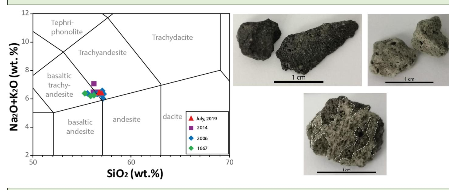
Microprobe analysis suggest that despite the similar whole-rock compositions, some compositional differences exist in the groundmass. Microprobe analyses indicate two types of glass in samples collected from the July 19<sup>th</sup> eruption; trachyandesite (UBI-19-03C) and rhyolite (UBI-19-03E). Glass from July 22<sup>nd</sup> (UBI-19-24A) suggest an intermediate composition between the other groups emitted during the previous days.
