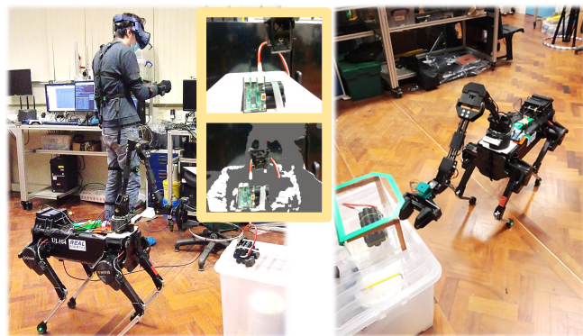
Fig. 1. Teleoperative legged manipulator system: a teleoperator with VR headset and wearable IMU-based motion capture, controlling locomotion and manipulation.
