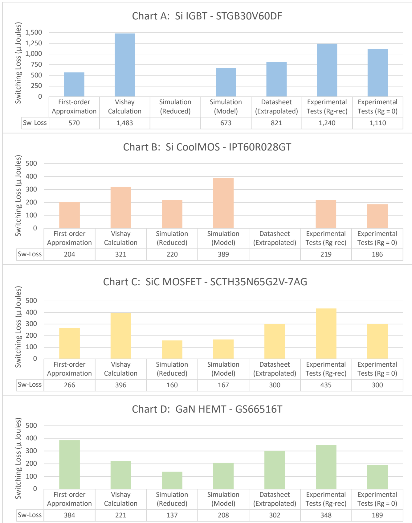
Figure 7: A comparison between switching energy loss evaluation methods and experimental test results from the switching circuits developed by the authors, in relation to accuracy. All with datasheet recommended R_g unless otherwise noted.
