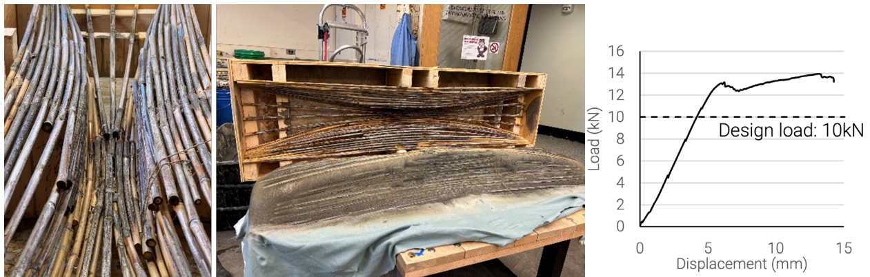
Figure 9: Formwork and casting of a 1m beam built using bamboo formwork and the load test results demonstrating ductile failure beyond the design load of 10kN.
