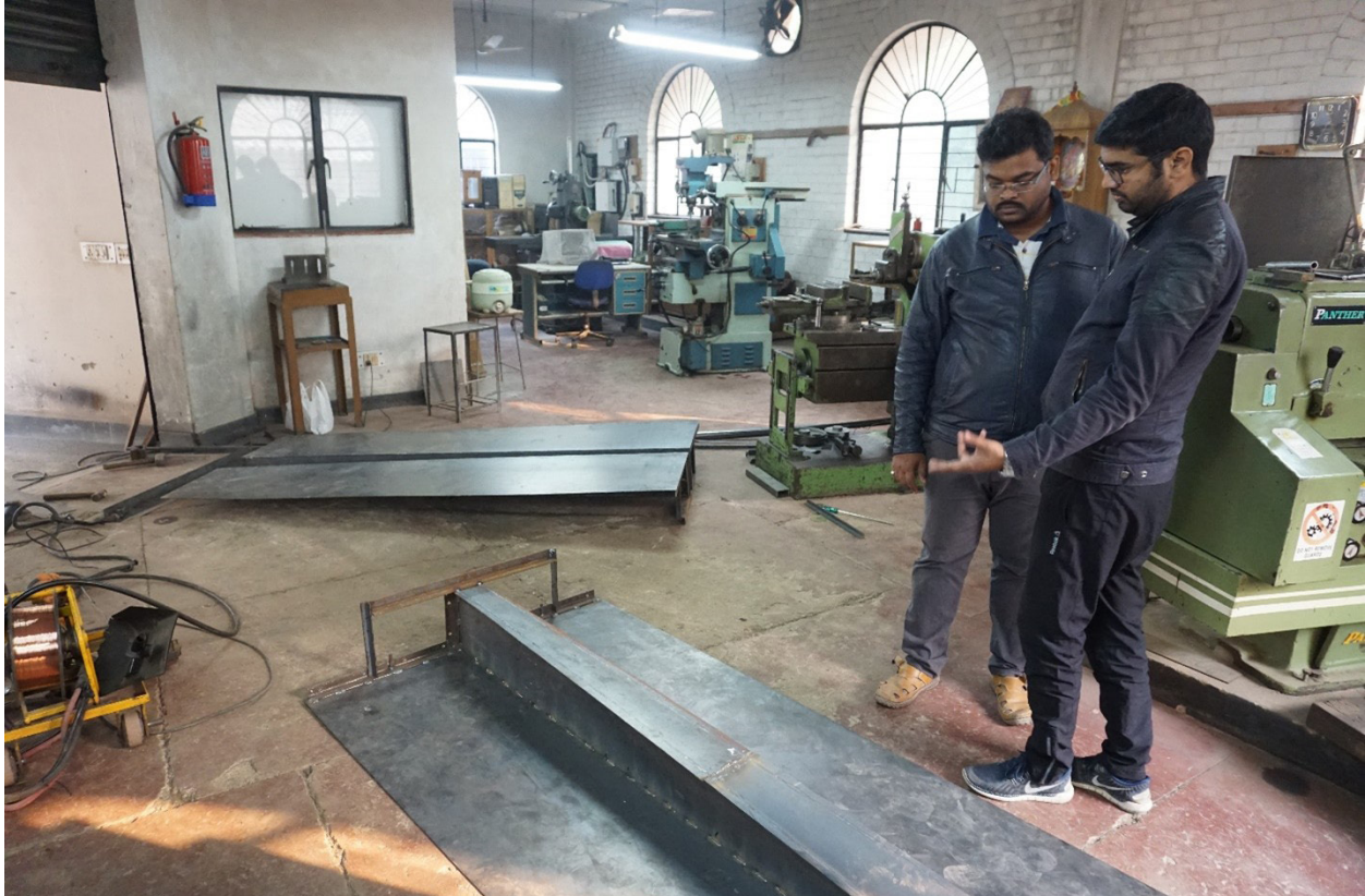
Figure 10: Steel plate formwork for a shaped concrete slab in New Delhi.
