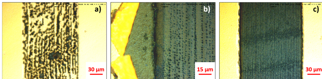
Figure 6. P3 laser ablation microscope analysis: (a) Optical image for a 130 \mu\text{m} width P3 scribe obtained by using a RSD of 3 \mu\text{m} and a pulse fluence value of 221.2 \text{ mJ}\cdot\text{cm}^{-2} . In this case, the presence of electrical bridges between module constituting sub-cells due to an incomplete gold removal is clearly visible; (b) Optical image for a 130 \mu\text{m} width P3 scribe obtained by using a RSD of 3 \mu\text{m} and a pulse fluence value of 354 \text{ mJ}\cdot\text{cm}^{-2} . In this case, the layer delamination on the edge of the ablated area is due to excessive stress experienced by the gold film during the P3 ablation; (c) Optical image for a 130 \mu\text{m} width P3 scribe obtained by using a RSD of 3 \mu\text{m} and a pulse fluence value of 306 \text{ mJ}\cdot\text{cm}^{-2} . The as-optimized P3 ablation resulted in an ablated area with negligible gold residual flakes and sharp edges without layer delamination.
