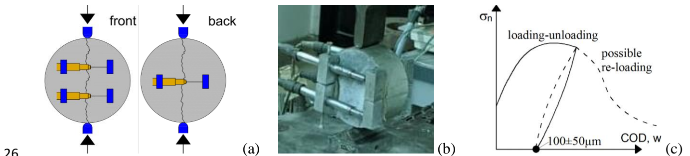
Figure 1. Pre-cracking of disks as implemented at PoliMi for chloride penetration and permeability tests: (a) front and rear views of the set-up, (b) picture of a test and (c) qualitative loading curve.
