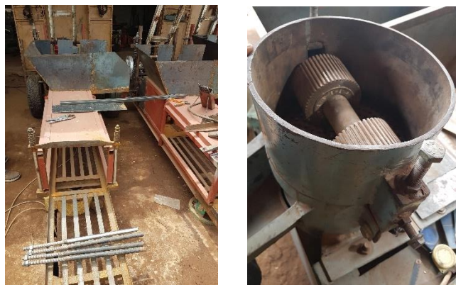
Figure 3: Locally produced straw bailer and pelletizer (U.Rudiger, 2023)
