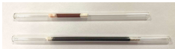
Figure 3. Samples of hematite (above) and charcoal activated powder were used as the adsorbents for radon in the air ( m = 0.3 \text{ g} ).
