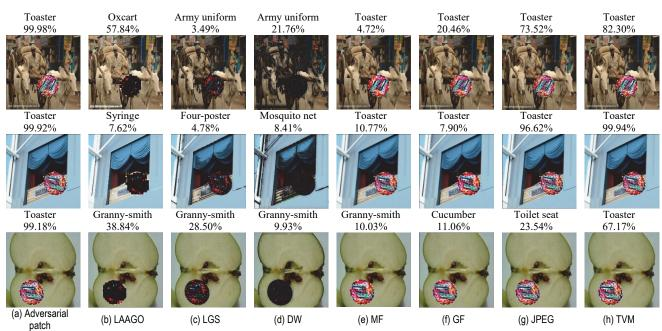
Figure 11 The Inception v3 confidence scores are shown on the example images. The images in the figure used the adversarial patch attacks, where (a) is the original adversarial sample, and (b) used the LAAGO algorithm. Columns c, d, e, f, g, and h list the results after LGS with λ equal to 2.3; DW, MF, GF, JPEG with quality 30; and TVM with weights equal to 10 processing, respectively
