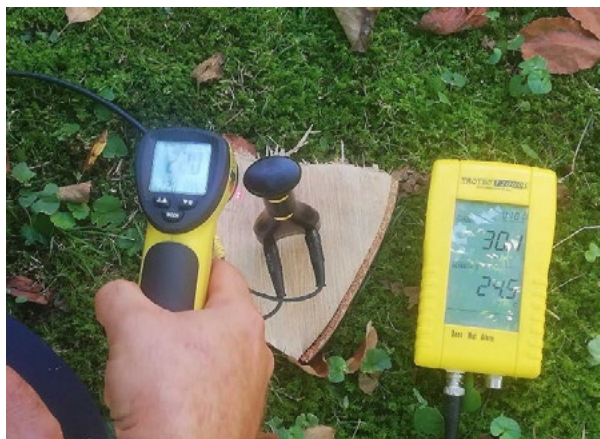
Figure 5: Moisture measurement of a fresh 30 mm section
