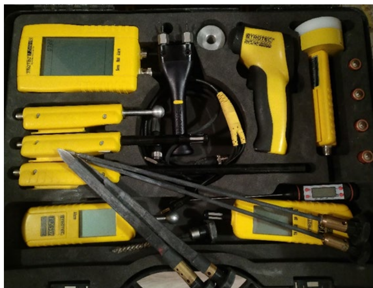
Figure 2: Measuring device Trotec T2000 with measuring electrodes and probes
