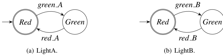
Figure 5.13: Traffic lights plant automata.
