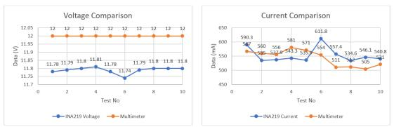
Fig. 7. Measurement comparison chart (a). Voltage (b). Current against the test number
