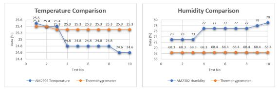
Fig. 8. Measurement comparison chart (a). Temperature (b). Humidity against the test number
