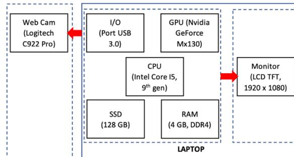
Fig. 4. Hardware design architecture
