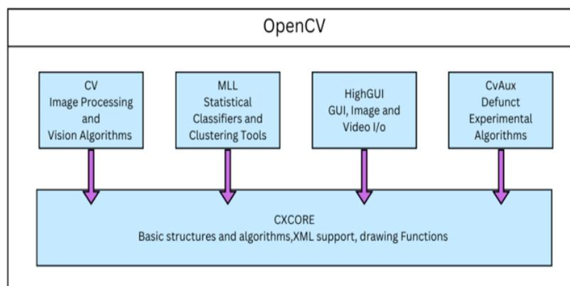
Fig. 3. The structure of OpenCV
