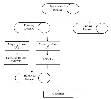
Fig. 3. Gaussian Based-SMOTE and SMOTE method Flowchart
