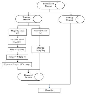
Fig. 2. Flowchart of the Gaussian Based-SMOTE method
