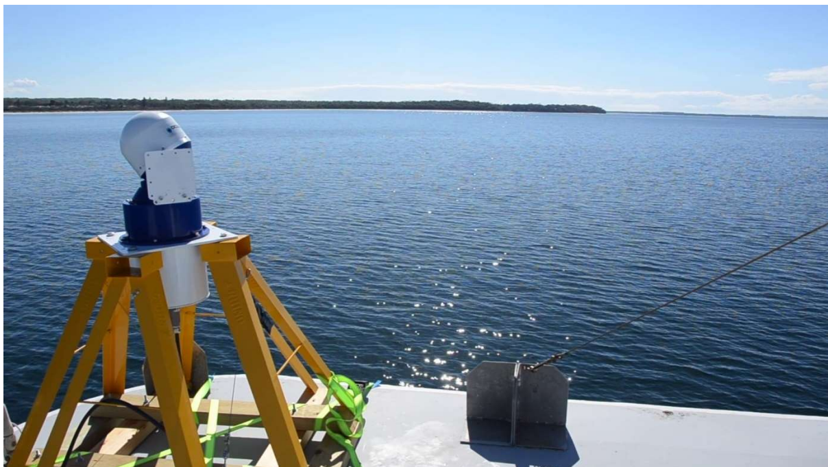
Figure 1. Setup of the Tau 2 integrated into the RobotEye on the top platform of a vessel operated by Dolphin Watch Cruises
