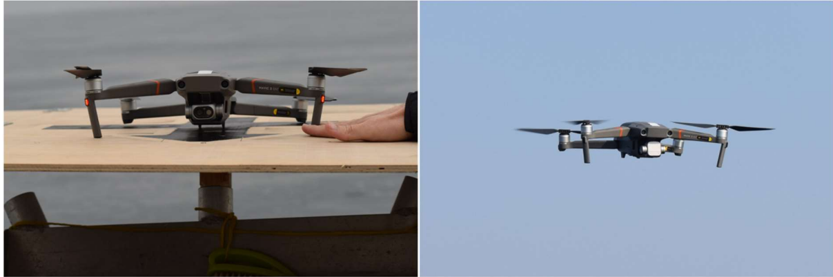
Figure 3. The DJI Mavic 2 Enterprise Dual on the launch pad at the stern of the boat (left) and in flight (right).
