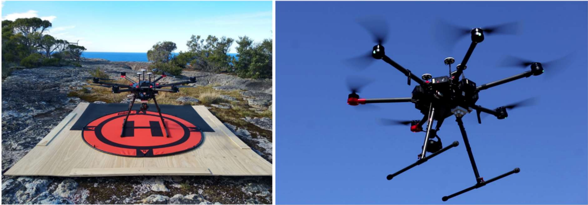
Figure 2. The DJI Matrice 600 Pro with mounted DJI infrared Zenmuse XT2 sensor shown on the launch pad (left) and in flight (right).
