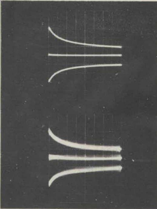
Fig. 5.43 1000 c/s ( m, H'' ) TRACES ILLUSTRATING THE NULL CONDITION FOR THE ADJUSTMENT OF H' IN THE MEASUREMENT OF THE ANISOTROPY TORQUE T(\theta) BY THE METHOD OF SECTION 5.4
