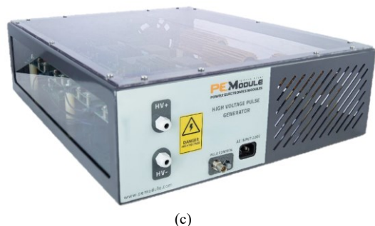
Fig. 5. Implementing a 4-module SMG (a) One module schematics. (b) One assembled module. (c) overall SMG with the associated casing.
