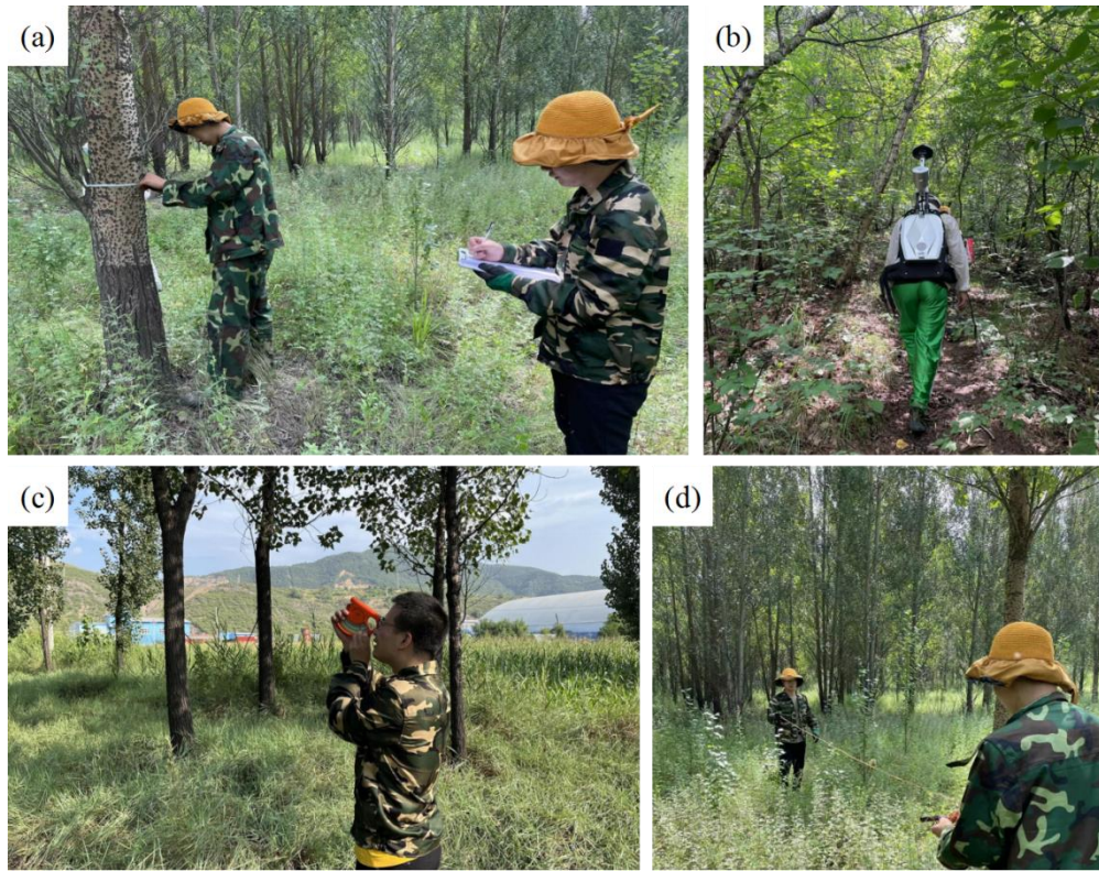
191 Figure 2. Forest sample plot survey (a) single tree diameter at breast height 192 measurement using a diameter at breast height ruler; (b) scanning the forest sample 193 plot using a backpack LiDAR; (c) single tree height measurement using a height 194 gauge; (d) measuring the extent of the forest sample plot using a measuring rope.
