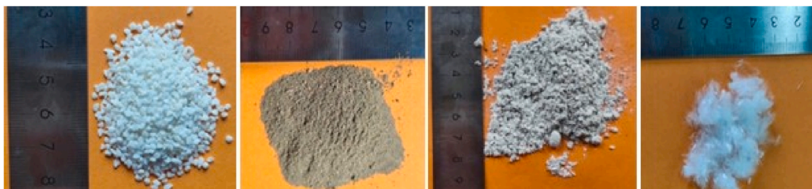
Fig. 3. Plugging materials used in the experiment (calcium carbonate, NT-DS, GT-MF, LCC-200 in sequence).
