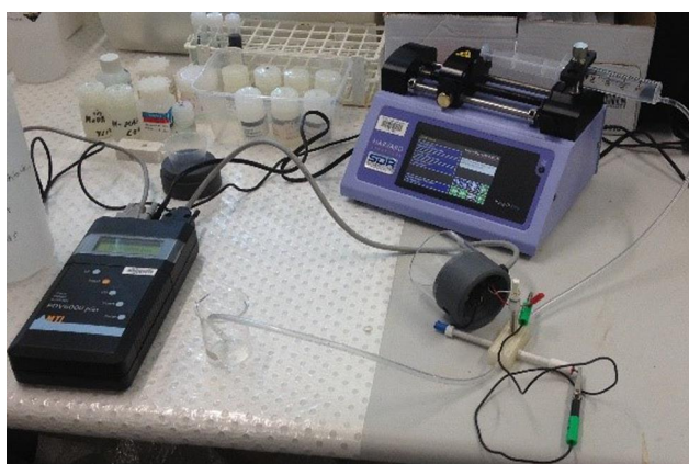
Fig. 6. Arrangement of the first ASV test conducted using the 3-D-printed device.
