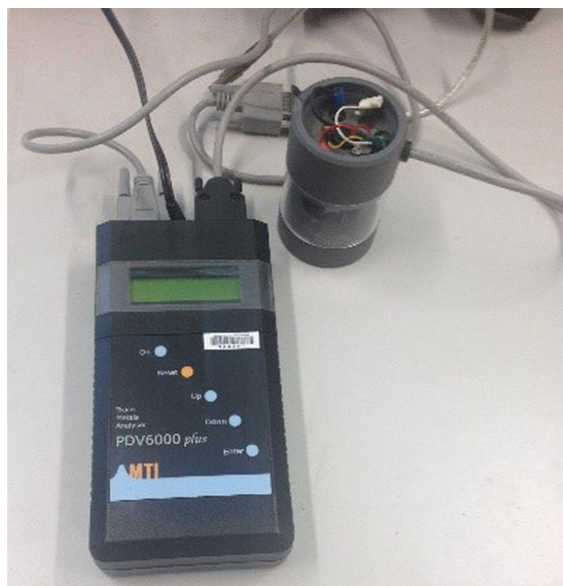
Fig. 2. PDV6000+ device used to validate the 3-D-printed device in its standard configuration.
