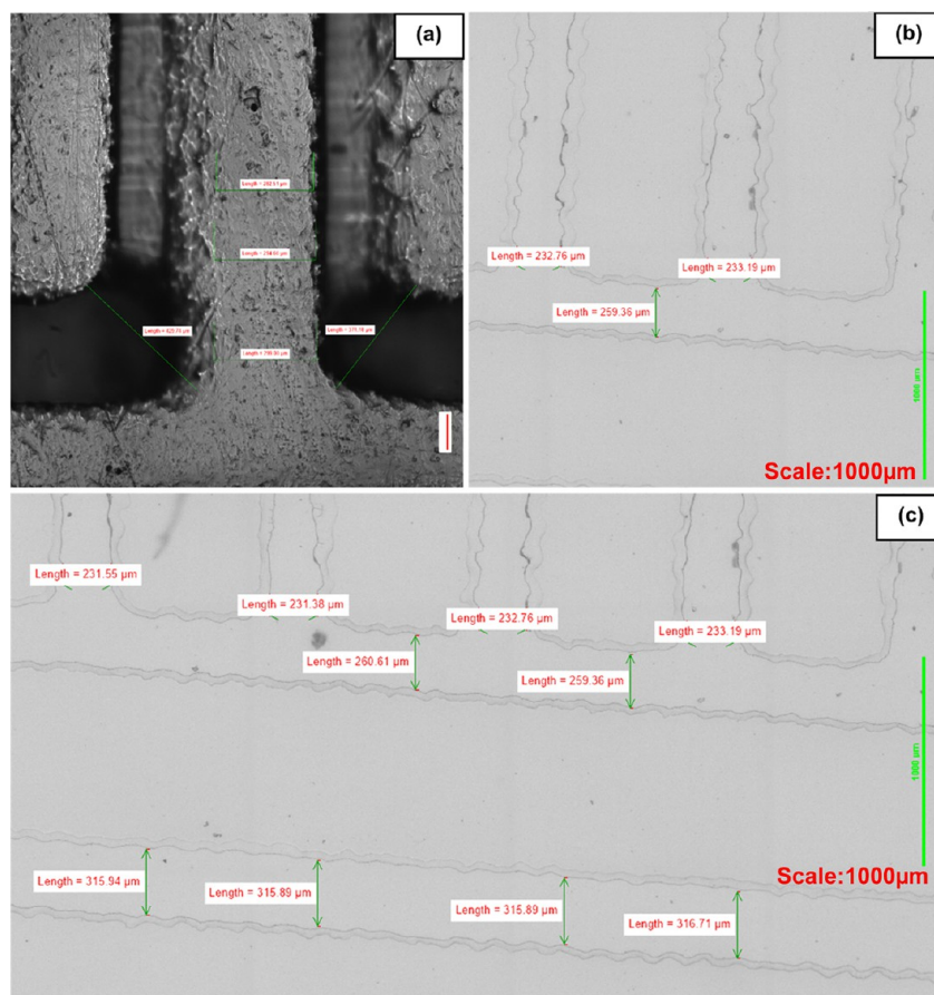
Figure 13. Comparison between 3D-printed (a) and homebrew-produced channels (b, c). Homebrew channels produced a flatter, more uniform surface and lower variation in dimensions than the 3D-printed counterpart, whose rough surface resulted in greater variability in channel walls. The consequent surface roughness of the 3D print was replicated by the PDMS chip which consequently failed to plasma bond to glass due to the uneven surface, (a) 282.51, 294.60, 429.74, 299, 371.18 \mu\text{m} , and (b) 232.76, 259.36, 233.19 \mu\text{m} , and (c) 231.55, 231.38, 260.61, 232.76, 259.36, 233.19, 315.94, 315.89, 315.89, 316.71 \mu\text{m} .
