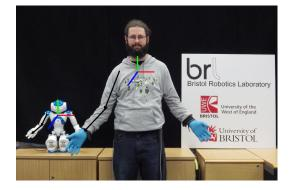
Fig. 2. A matched pose between the tele-operator and the NAO robot. The directions of the arm unit vectors are indicated with black arrows, torso coordinate frames in RGB (XYZ).
