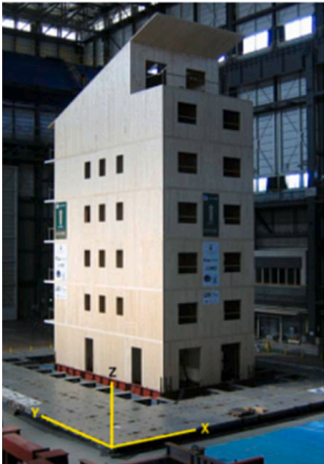
Fig. 6. The 7-storey CLT structure in SOFIE project [14].
