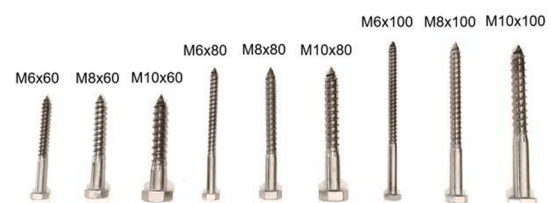
Fig. 3. Coach screws used in cyclic tests.
