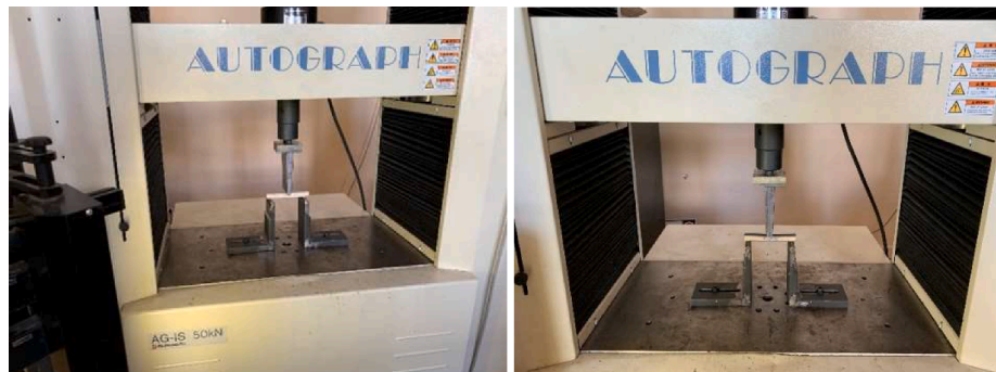
Fig. 5. Three-point bend tests for balsa and sandwich samples.
