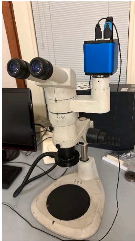
Fig. 4. The image of the stereo microscopy setup.
