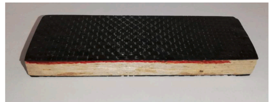
Fig. 3. Detailed image of the sandwich sample.
