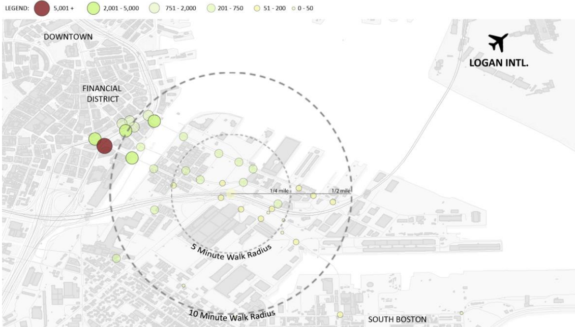
Figure 6: Pedestrian volume by intersection for the peak hours. Source: authors’ elaboration based on the South Boston Waterfront Sustainable Transportation Plan 2015 .
