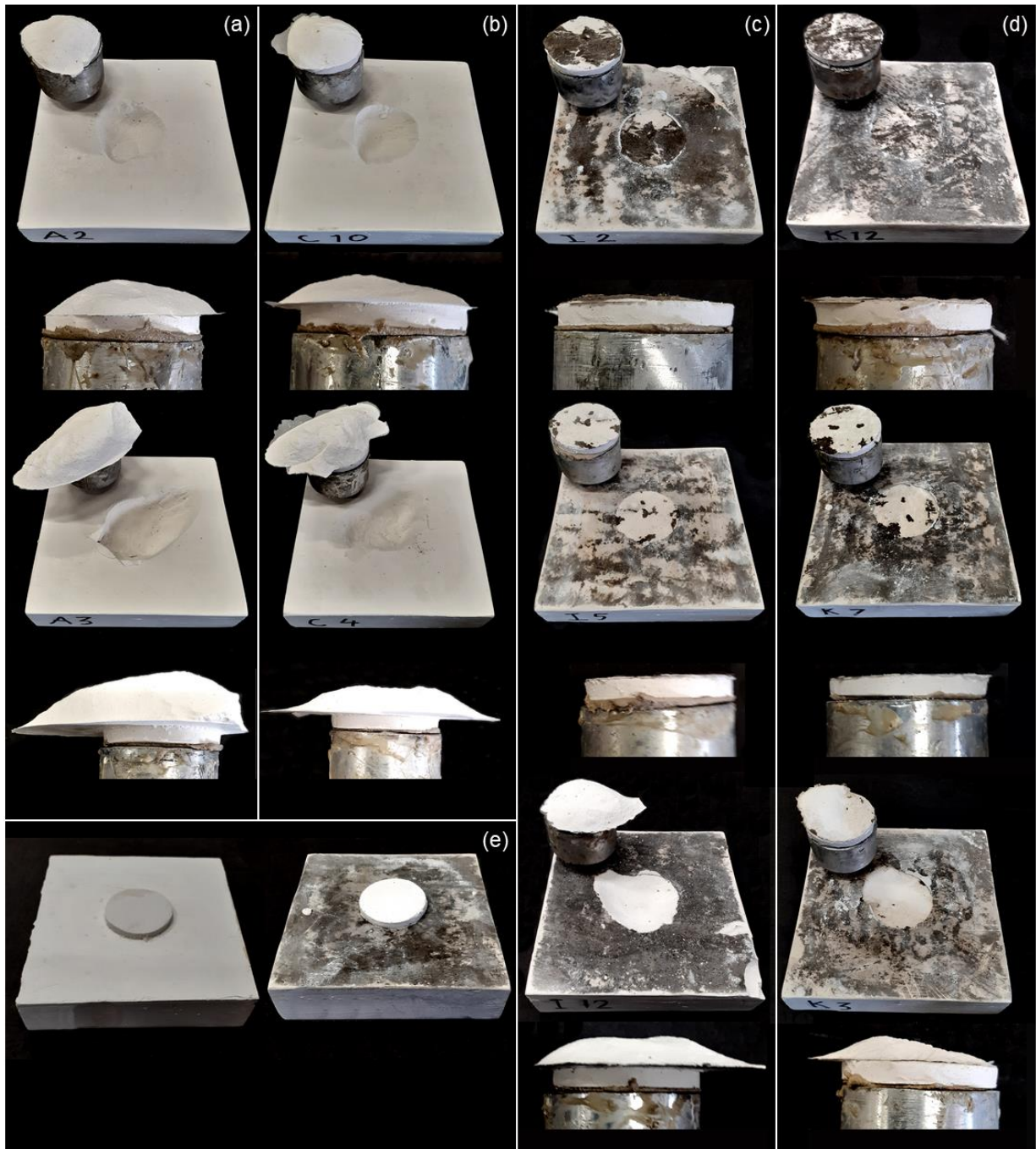
594 Figure 9 - Tested specimens from groups AP-CB, AP-QF-CB, AP-DB, and AP-QF-DB. (a) Group AP- 595 CB, cohesive failure of base material. (b) Group AP-QF-CB, cohesive failure in bases. (c) Group AP- 596 DB, partial cohesive failure of base material (top, middle) and cohesive failure (bottom images). (d) 597 Group AP-QF-DB, partial cohesive failure of base material (top, middle) and cohesive failure of base 598 material (bottom). (e) Clean based (left) and dirty (right) specimens. Cylinders 50 mm Ø and base 599 dimensions 150 mm x 150 mm.
