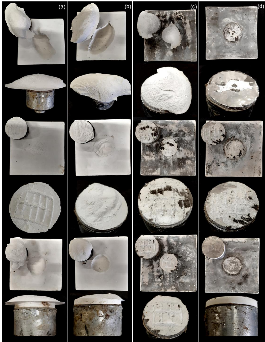
611 Figure 11 - Tested specimens from groups J-CB, J-QF-CB, J-DB, and J-QF-DB. (a) Group J-CB, 612 cohesive failure in the base (top and lower) with one exception of largely adhesive failure where 'keying' 613 is evident (middle). (b) Group J-QF-CB, cohesive failure in base material. (c) Group J-DB, cohesive 614 failure (top) and partial cohesive failure of base (middle, lower). (d) Group J-QF-DB, partial cohesive 615 failure of base material (top, middle), adhesive failure (lower). Cylinders 50 mm Ø, base dimensions 150 616 mm x 150 mm.
